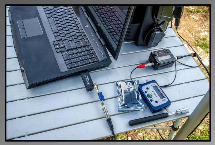
SDR Dongle plugs into Laptop or Computer. Other end plugs into the second Connector on the LNB.
